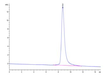
The purity of Mouse uPAR isoform 1 is greater than 95% as determined by SEC-HPLC.
